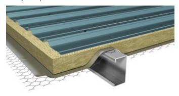
Double Skin Metal Deck Roof - Corrugated or profiled top metal sheet fixed to the bottom corrugated metal sheet using a spacer system which is then fixed onto the purlin. This roof construction typically uses mineral fiber as insulation.
